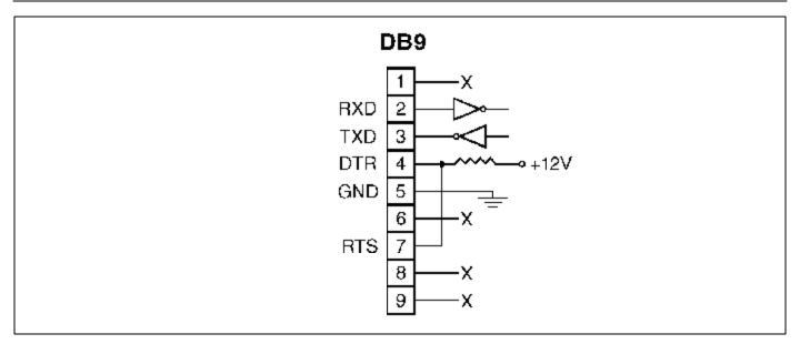
Figure A.1: Console Port Interface (DTE)
